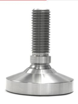
Stainless steel articulated feet designed in order to obtain the best weighing performances, particularly suitable for creating scales with 4 load cells. Extremely compact and easy to install, the feet minimize the height of the platform and ensure a perfect decoupling of the lateral forces during the weighing operation.
